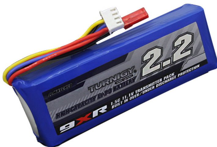
Figura 27: Li-Poly, 11.1v (3s) 2200mAh 1.5C fornecida pela HobbyKing.
